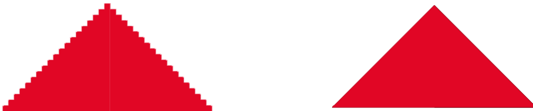
Raster image showing stairstepped pattern of "on - off" pixels along the diagonal.
